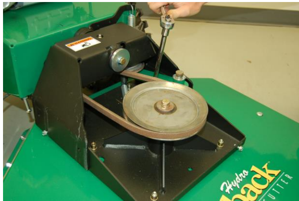
Removing tension on the blade belt
