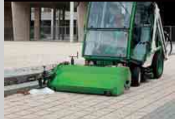
Sweeper with box and gutter brush
