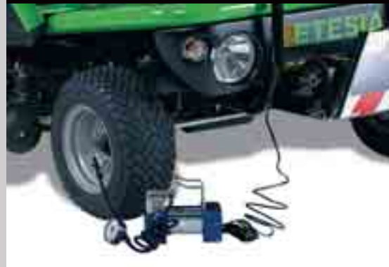
12 Volts electrical socket
