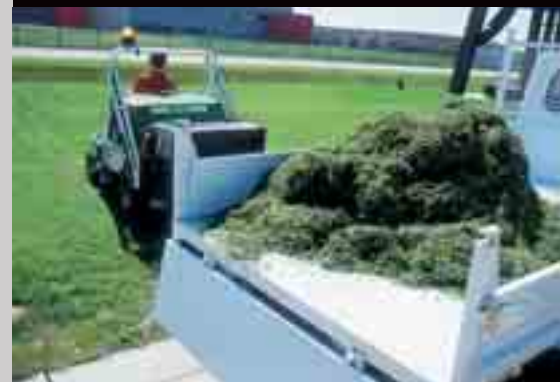
Grassbox emptying up to 1.80 m height (h124D and DX models)
