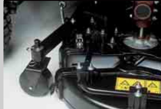
Cutting deck is removable without the use of tools (h124D model & h124 DX model)
