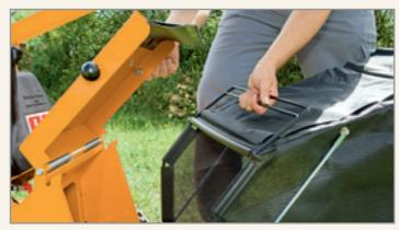
Model AS 530 MK is equipped with a low-wearing and easy-to-maintain blade clutch. This function allows transportation between sites without fear of blade damage or objects being thrown out. Or simply empty the collecting bag without any need to restart the engine. Any danger is completely eliminated, as the blade stops immediately.
